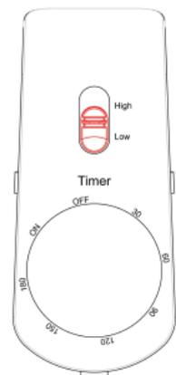
**IMPORTANT:** Never turn the switch clockwise further than "180" (resistance can be felt). Otherwise the switch will break! Do the same anti-clockwise: Never turn beyond the "On" position!
